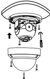
5. Adjust the monitoring direction of the lens (tighten screws after vertically adjusting the lens).
