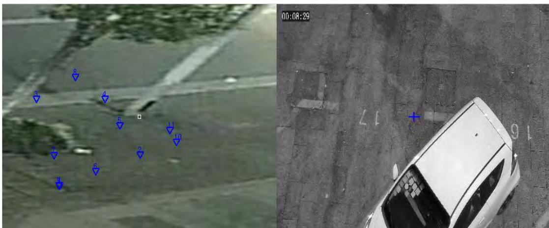
8. Turn the slave camera to the position where the marking point is. Set the magnification of the slave camera to the maximum, and make the cross in the center of the slave camera image coincide with the marking point (the small white frame) in the master camera image. Click **OK** and **Orient** to link the marking points. Click **Cancel** to cancel the linked marking points.
