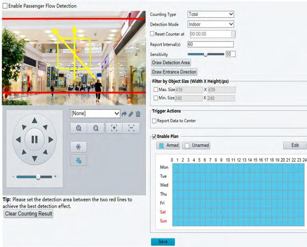
2. Select **Enable Passenger Flow Detection**. Select a detection mode, set report interval and sensitivity.
