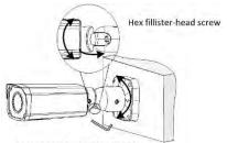
Loosen two hex fillister-head screws using a 4# hex I-key (that should be purchased separately) to avoid damaging the universal joint. Then adjust the camera to the desired monitoring direction. Fasten the screws to finish.
